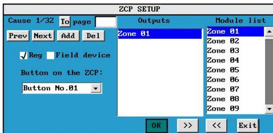
There are 32 default configurations for each unit of LEDs with a button. Similar to the left, register the default setting so that each unit corresponds to a unique zone as it defines.
