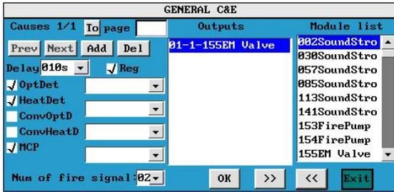
The meaning of this c&e is when any 2 of smoke detector, heat detector or manual call point are active, the electromagnetic valve wired after the I/O module with the address of 155 will be triggered after 10s.
